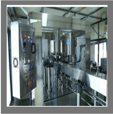
90 BPM Rinsing, Filling and Capping Plant
